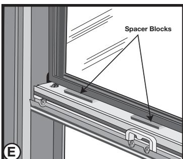
**STEP 5.** Replace the Interior Vinyl Glazing Beads. Start with the TOP piece, bottom piece next and then side pieces. Insert the shorter leg of the glazing bead into the glazing groove, starting at one end. Press it in until it snaps into place along the entire piece. Be careful to not damage glass or the bead.
