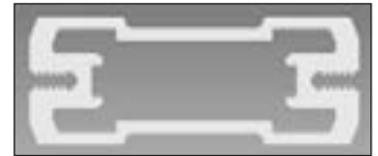
(1) Aluminum mill structural tube mull
